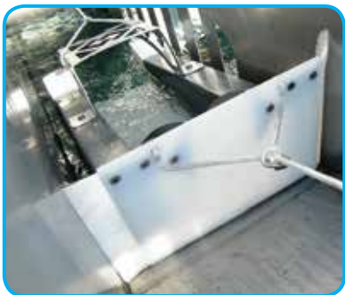
Self-adjusting grease scraper with limited water removal
