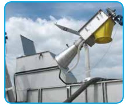
Easy maintenance thanks to wide inspection hatches
